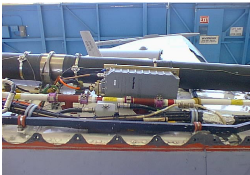
Figure 12. GAS-1N AE Mounted below Panel #40
