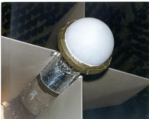
Figure 11 Mini-array mounted on Boeing PGM tailkit.
